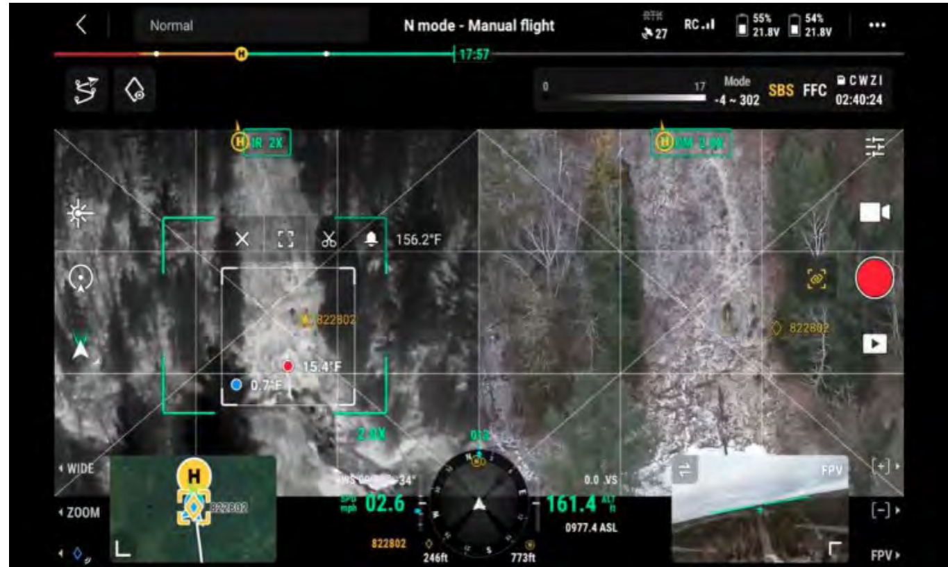
Screenshot from a drone flight over an exposed natural gas pipeline on Reservation, showing both an aerial and white-hot thermal image side-by-side. Thermal imaging is showing a temperature difference between the pipeline and the surrounding area. (Bad River Tribe, Will Affect Letter, Figure 13)
